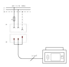
H 2 P for 230 V with power supply 230 V / N / PE / 50/60 Hz, connected through 3-pole shock-proof (Schuko) plug system.
